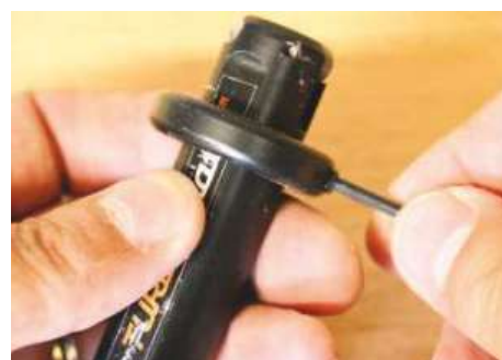
▲ The collar can be used to restrict the plunge depth of the tool
